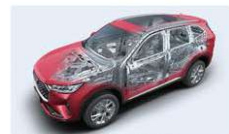
71.61% high-strength steel body
